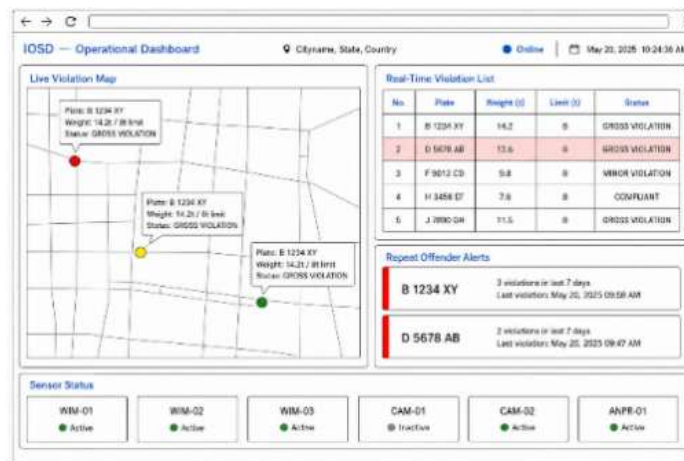
Figure 4. Wireframe of the IOSD Operational Dashboard for Field Officers at UPPKB Weighbridge Stations
